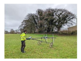
Bartington Grad 601-single axis dual sensor gradiometer.
